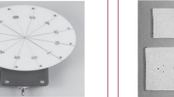
The Model L-629 Rotating Spoke Test Tool is used to evaluate the performance of fluoroscopic imaging systems. The tool demonstrates screen image lag, motion blur, contrast, and related distortions encountered in fluoroscopic examinations. (per AAPM Report #60)
